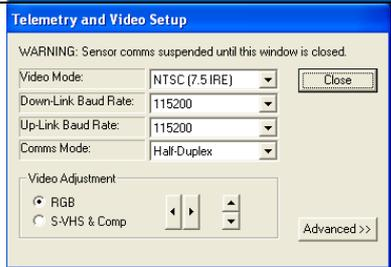
Changing Baud rate Using sonar control software
