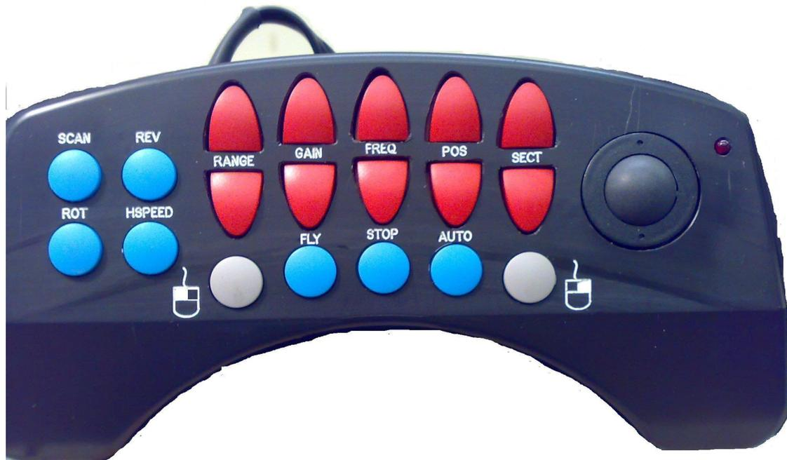
Remote controller will be hooked to front panel connected to PS/2 using curly cable. It should be always be connected to PS/2 .
