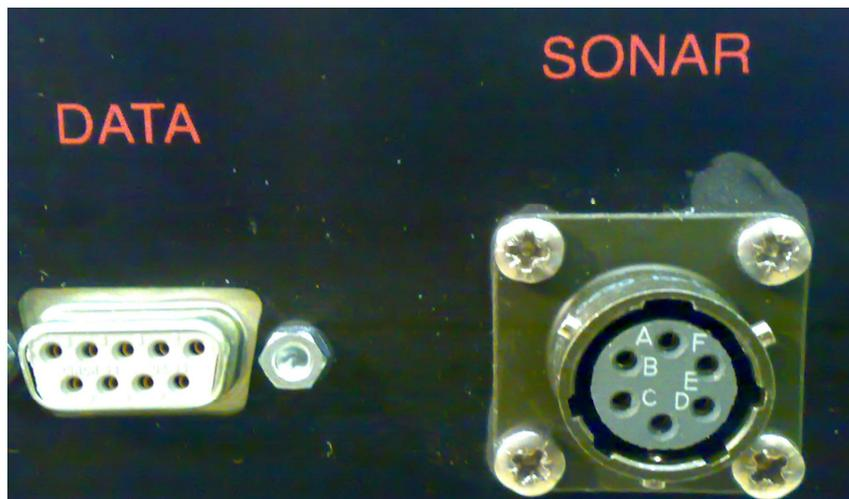
Connection to the sonar is made via a 6 pin ITT cannon connector(SONAR) or 9 pin D type situated on the rear of the unit.
